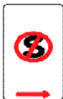
No stopping sign
